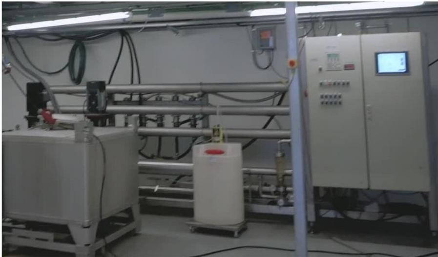
**Demonstration scale Nano filtration plant (100 m<sup>2</sup>)**
