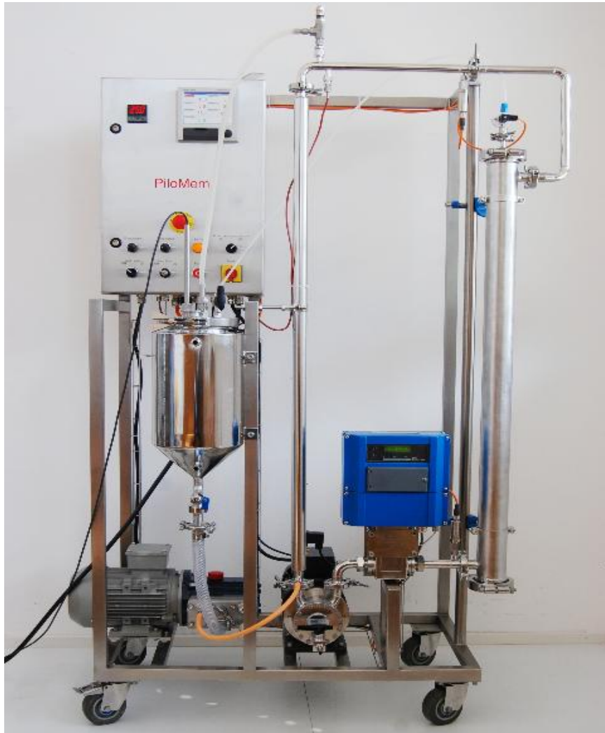
PILOT SCALE NF PLANT OF 2,6 m 2 FILTRATION AREA FITTED WITH GE HL MEMBRANE
